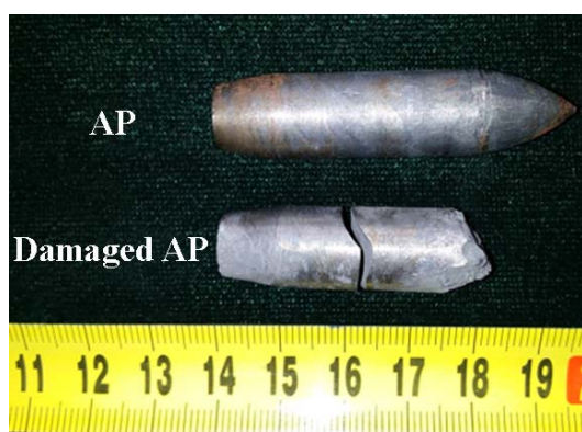
图 20 穿甲弹侵彻靶体后毁伤状况 Figure 20 Damage and failure of the AP projectile after DOP test
