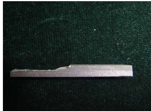
图 13 层状复合材料三点弯曲测试失效样品 Figure 13 The failed samples of the laminated composite after 3-point bending test
