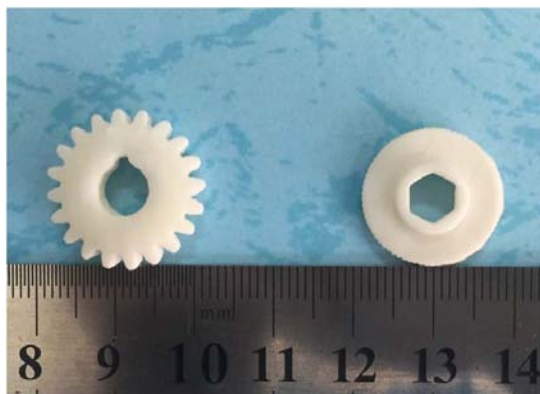
图 12 光固化增材制造的 ZTA 陶瓷制件 [69] Figure 12 ZTA ceramic parts with the stereo lithography apparatus [69]
