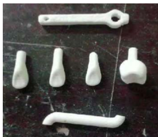
图 5 SLS 工艺成型氧化锆陶瓷零件 [14] Figure 5 Zirconia ceramic parts fabricated by SLS [14]
