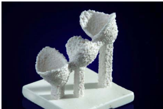
图 7 SLM 工艺成型的陶瓷件 [15] Figure 7 Ceramic parts manufactured by SLM [15]
