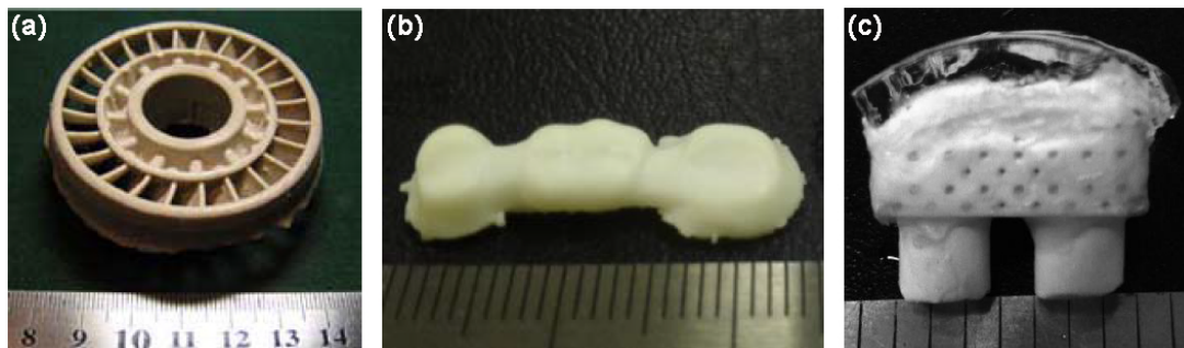
图 12 光固化成型陶瓷制件: (a) 二氧化硅叶轮 [21] ; (b) 氧化锆牙桥 [24] ; (c) 骨软骨组织工程支架 [26] Figure 12 Ceramic part fabricated by stereolithography: (a) silicon dioxide impeller [21] ; (b) Zirconia dental bridge [24] ; (c) osteochondral scaffold for tissue engineering [26]
