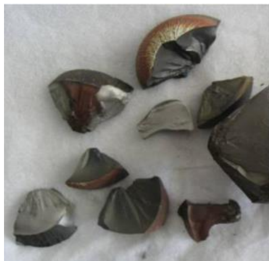
图 7 ZrB_2-SiC 陶瓷材料在高频等离子体风洞烧蚀试验后的照片 Figure 7 Photographs of ZrB_2-SiC UHTC after high-frequency plasma tunnel ablation test
