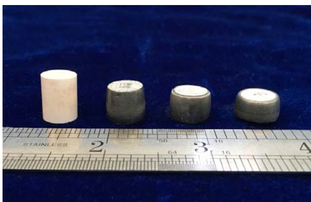
图 1 试样超塑性压缩变形前后的典型形貌 Figure 1 Typical images of the specimens before and after superplastic compression
